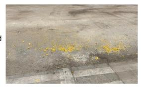
6/20/23 Slip & Fall injury on the hydraulic film present on the cone pocket floor. This hazard was generated by an earlier hydraulic oil leak from the deck compressor to the cone pocket floor. The oil leak was cleaned up. However, an oil film remained on the cone pocket floor and a worker slipped and fell. Causal factors: 1) Inadequate cleanup of hazard created the slippery conditions. 2) The slippery cone pocket floor was not observed before cone pocket use.
