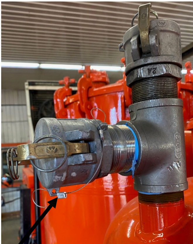
Wire Lanyard securing the cam-lock cap
