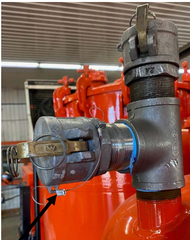
Wire Lanyard securing the cam-lock cap.
