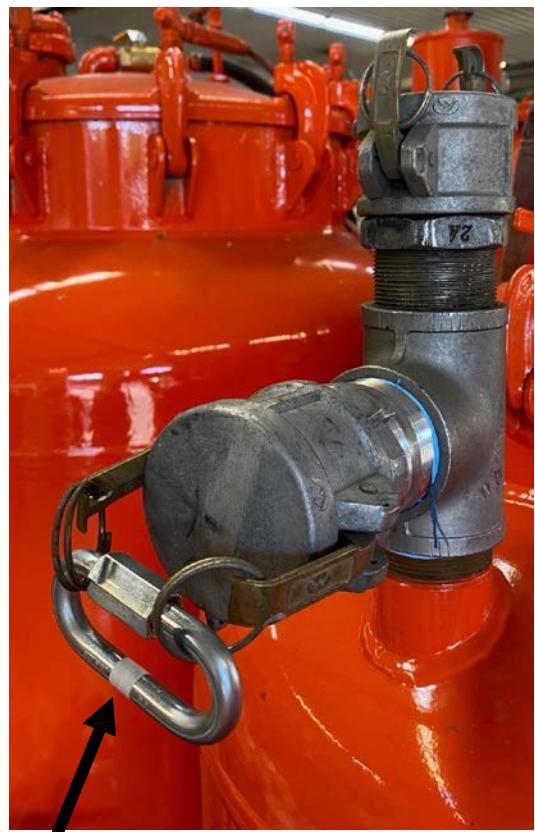
Oval Threaded Link securing the cam-lock cap.
