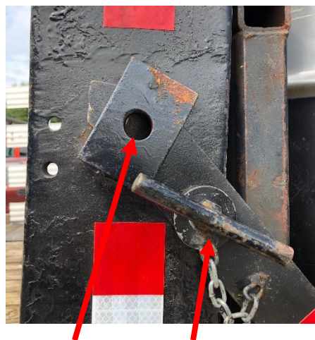
Latch Pin & T-Bolt Secure the Horizontal Safety Bar
