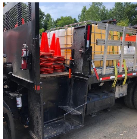
Coning seat ready for use. All safety supports are in place.
