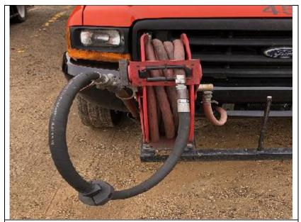
**Correct** – This truck is equipped with a holster for the air wand to go into. Notice that the hose is not kinked and the wand is secure in the tube holding it.
