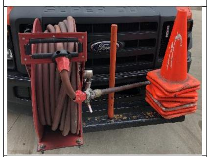
Incorrect – If the truck is not equpped with a holster do not secure the air wand by wedging it when not in use. Storing the hose in this manner weakens the hose where it bends at the coupler shortening the hose life and insreasing the risk of the wand becoming dislodged and dragging on the ground when traveling.
